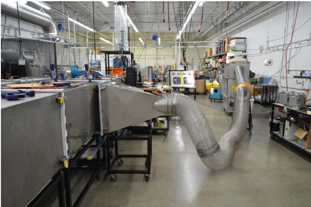
Figure 3. Cabinet door connected to laminar flow element.
